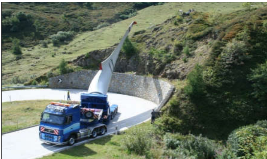
Plate 4-6 Blade Adaptor Transport System
